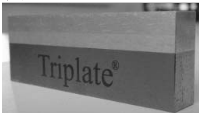
Fig 5: Triplate consists of a sandwich of three metals
