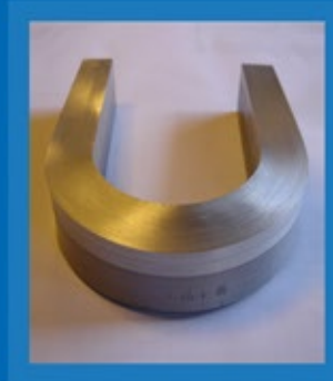
Bend test of Triplate
