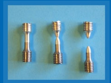
Tensile test of Triplate
