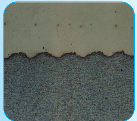
Interface Titanium / Steel 200x magnified
