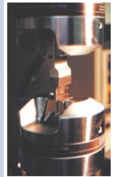
Through thickness tensile test of Triplate
