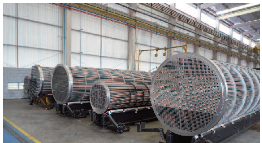
Fig. 2. Heat exchangers with a clad tube sheet (Photo by SMT b.v.).
