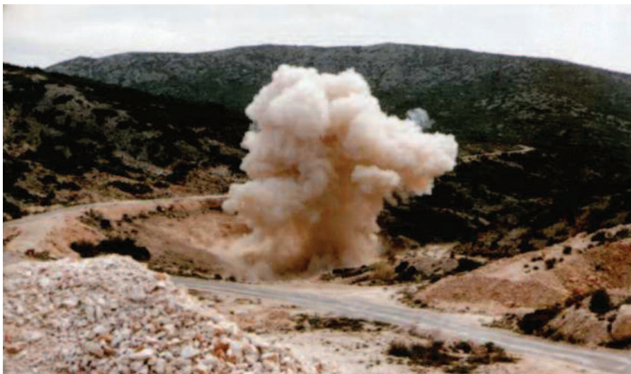
Fig. 1. Explosive cladding in the open air; also called atmospheric cladding for the sake of convenience (Photo by Innomet b.v.).
