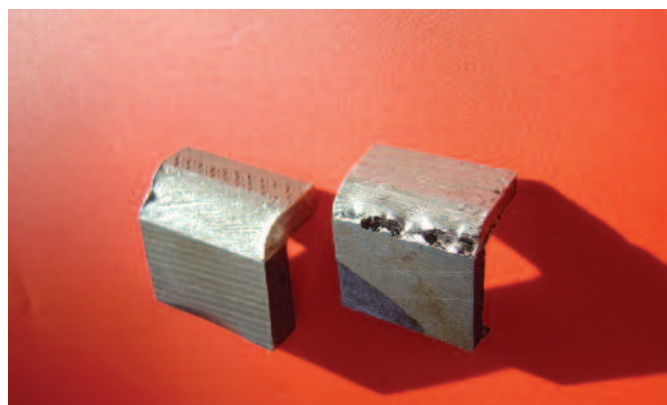
Fig. 7. The consequences of the 'Hammer Bend Test'. On the left is a vacuum cladding and on the right a cladding produced in the open air. The oxide conglomerates open out as a result (Photo by Innomet)
